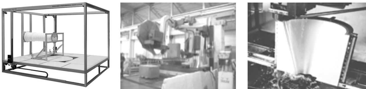
Figure 6. A computer controlled hot-wire foam cutter (left), a robotically controlled stone saw (middle) and a metal forming Wire-EDM machine (right) can generate ruled surfaces with straight cutting tools. In this way foam cast concrete, stone and metal details all share a similar formal logic.
